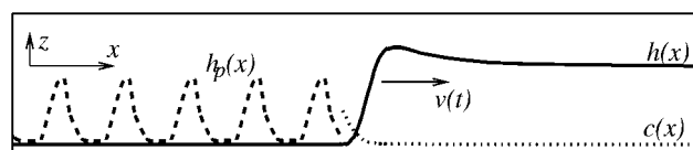
Fig. 1 Diagram showing a liquid front that recedes due to evaporation and convection. The front has varying velocity v(t) and the liquid film thickness profile is given by the function h(x, t) . In the bulk film the profile c(x, t) is the vertically averaged solute concentration profile and outside the liquid film, the solute layer thickness is given by h_p(x, t) = c(x, t)h(x, t) .
